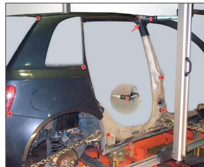
Pull accurately the first time, every time. Calipre's distinctive measuring system clearly displays necessary pull direction and travel length. Measuring reference points on Autorobot datasheets (some shown here in red) have all three length, width and height values. When all measurements have been pulled within accepted tolerance, with the help of the Calipre and datasheets, replacement parts fit accurately and the vehicle is restored to original condition.
