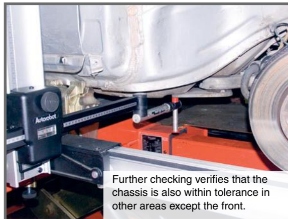
Measuring shows that the McPherson upper end has been pushed back by 4 mm and 2 mm to the side.
