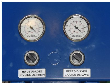
Simple On/Off function with vacuum gauges
