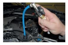
Removal via suction lance into the recovery tank
